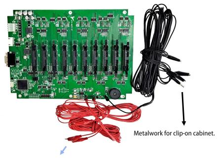
Signal wire for clip-on coin acceptor.
