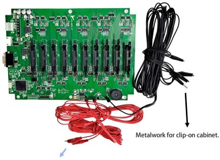
Signal wire for clip-on coin acceptor.
