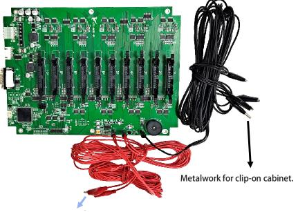
Signal wire for clip-on coin acceptor.
