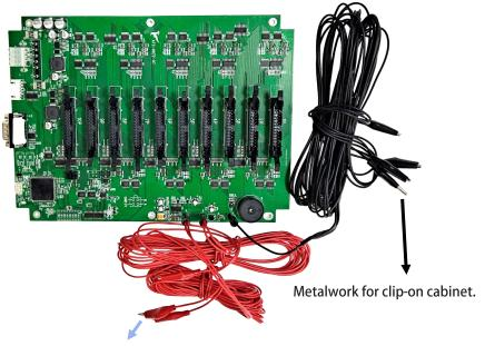
Signal wire for clip-on coin acceptor.
