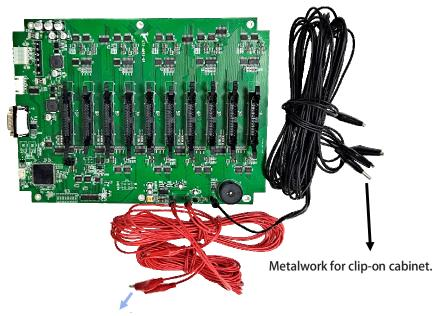
Signal wire for clip-on coin acceptor.
