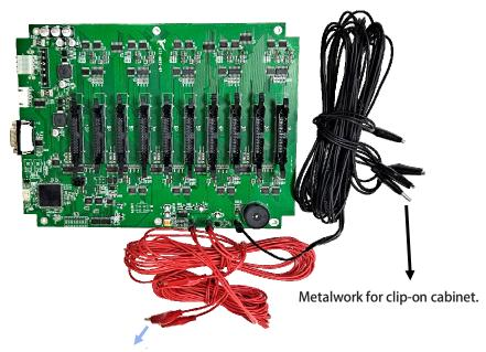
Signal wire for clip-on coin acceptor.
