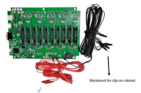
Signal wire for clip-on coin acceptor.
