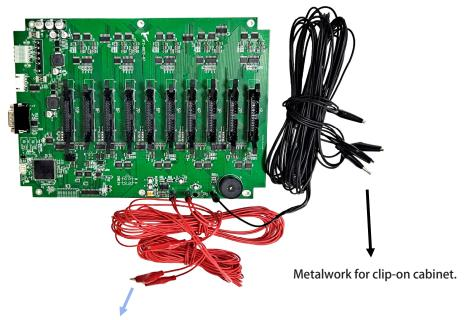
Signal wire for clip-on coin acceptor.
