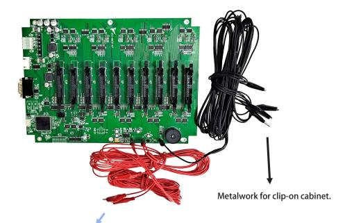
Signal wire for clip-on coin acceptor.
