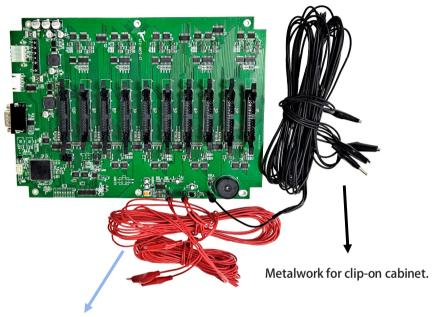
Signal wire for clip-on coin acceptor.
