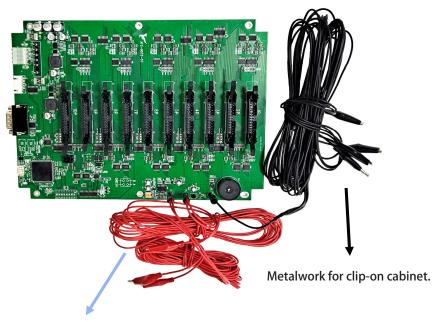
Signal wire for clip-on coin acceptor.
