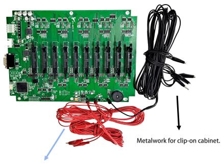
Signal wire for clip-on coin acceptor.
