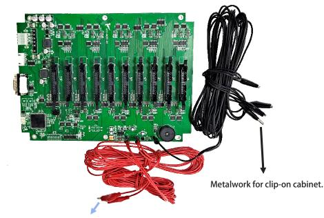
Signal wire for clip-on coin acceptor.
