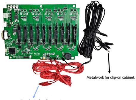
Signal wire for clip-on coin acceptor.
